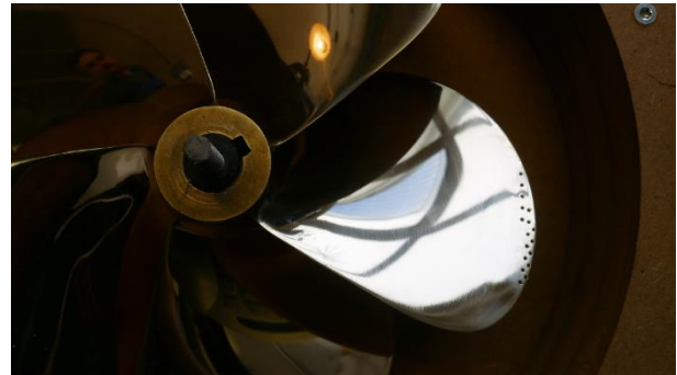
Figure 17 PressurePores™ as applied on the Princess Royal propeller for Modified Propeller-2
