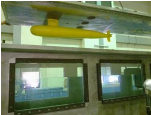
Figure 3 The dummy model of submarine is placed at the lid of the measurement section window
