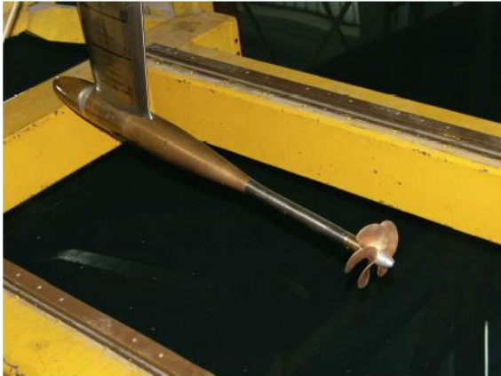
Figure 19 Towing tank open water test set-up
