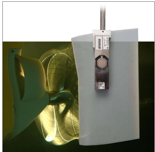
Figure 11 Montage Explaining the Concept for Rudder Resistance Measurement
