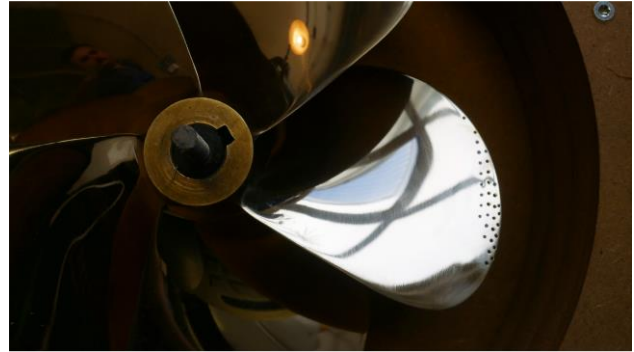
Figure 16 PressurePores™ as applied on The Princess Royal propeller for Modified Propeller
