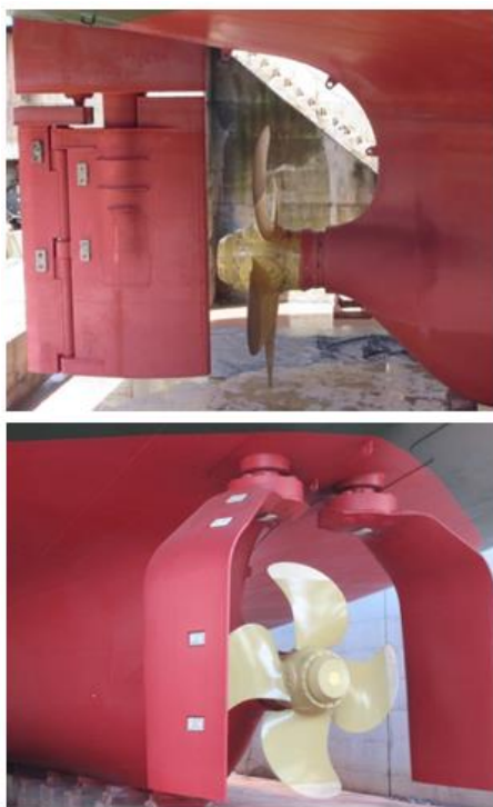
Figure 1. Conventional Flap-Rudder (Top) vs. GATE RUDDER® (Bottom).
