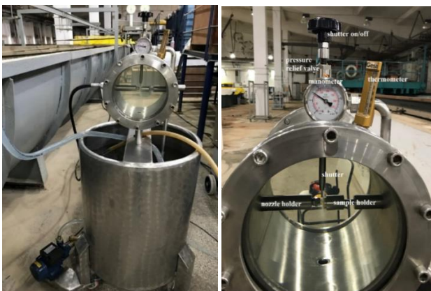
Figure 1 The water jet test rig and the cavitation chamber
