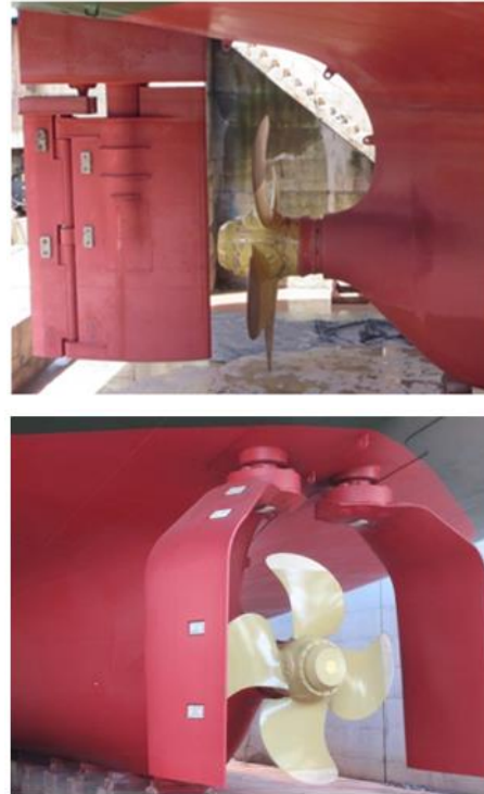
Figure 1 Conventional Flap-Rudder (Top) vs. GATE RUDDER® (Bottom)
