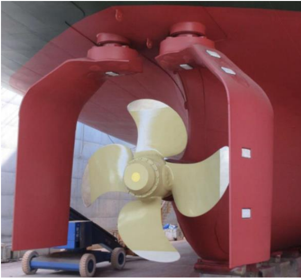
Fig. 1. Shigenobu, the first Gate Rudder System fitted ship
