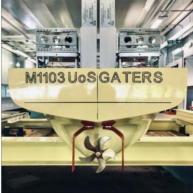
Figure 2 Rudder load measurement system.
