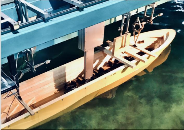
Figure 1: Resistance tests with a single-component electronic resistance dynamometer (OPN500).
