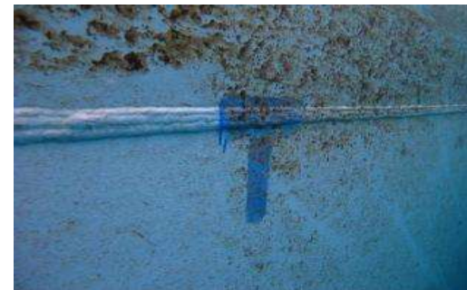
Intersleek®1100SR (left) on LNG carrier after 25 months compared to Intersleek®700 (top) and Intersleek®900 (right)
