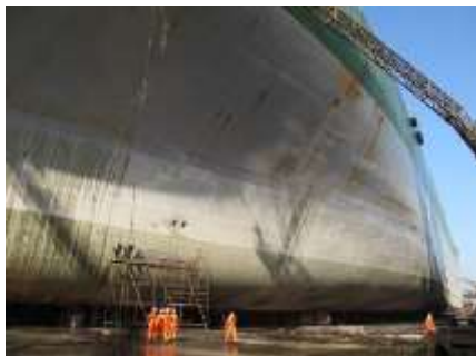
Intersleek®700 on VLCC after 60 months
