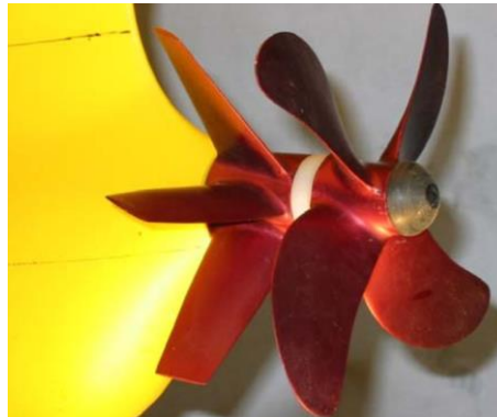
Biased Pre-swirl Stator Attached to 300K KVLCC model (Pusan University)
