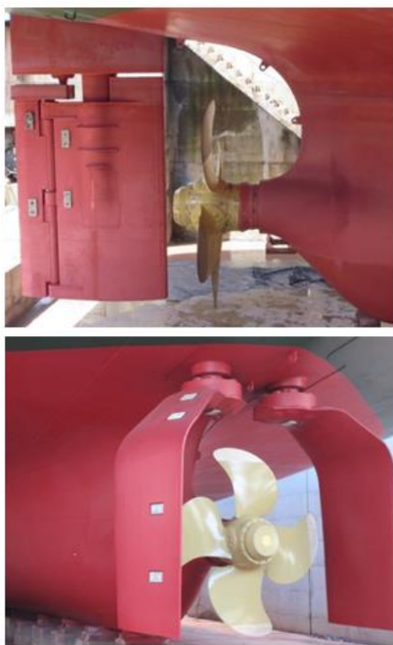
Figure 1. Conventional Flap-Rudder (Top) vs. GATE RUDDER® (Bottom).
