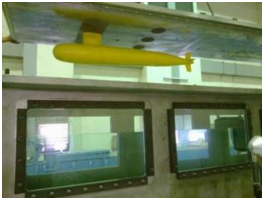
Figure 3 The dummy model of submarine is placed at the lid of the measurement section window
