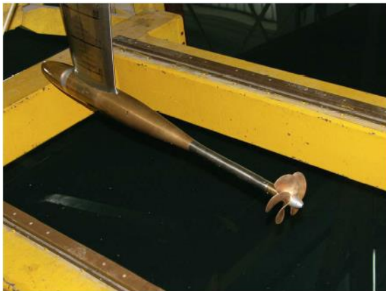
Figure 19 Towing tank open water test set-up
