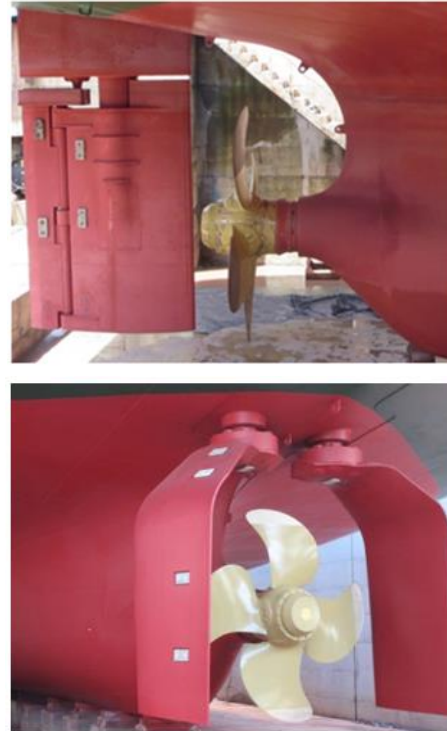
Figure 1 Conventional Flap-Rudder (Top) vs. GATE RUDDER® (Bottom)
